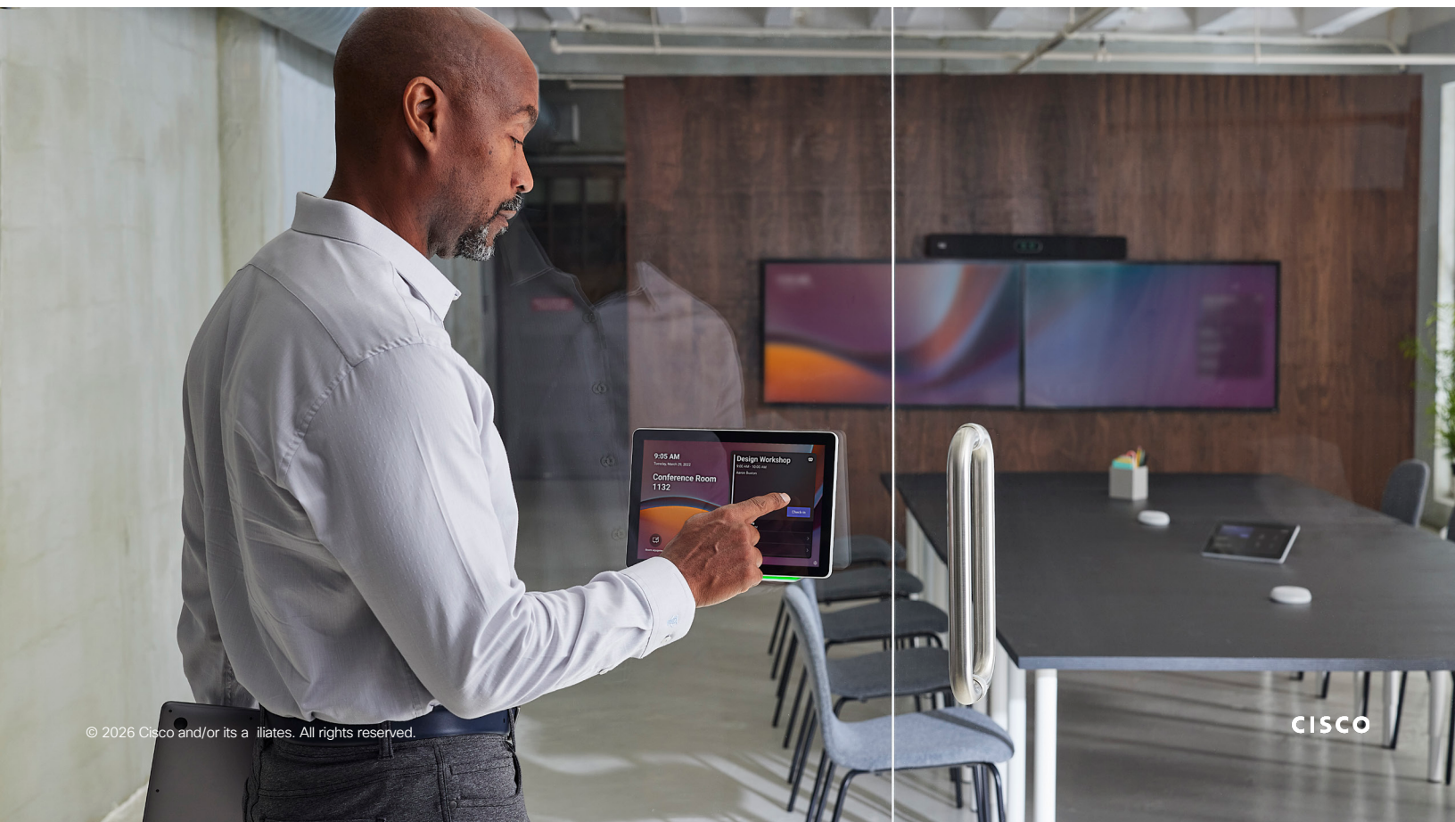
Figure 2: Cisco Room Navigator mounted on glass wall, running the native Microsoft Teams panel application
